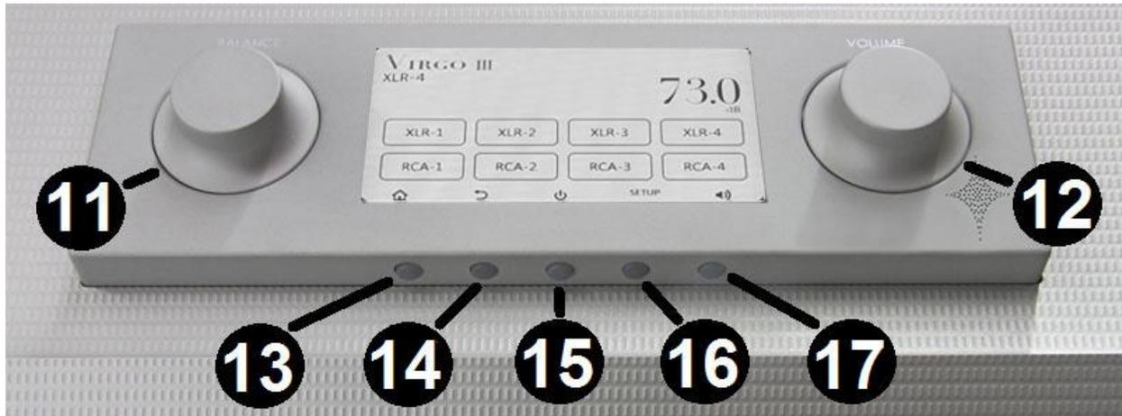
The front panel includes an LCD touchscreen and two knobs plus five buttons positioned underneath the display. These buttons allow you to control the Virgo III without its remote. The functions of the buttons are shown using icons on the Here are the functions of the buttons and knobs:
